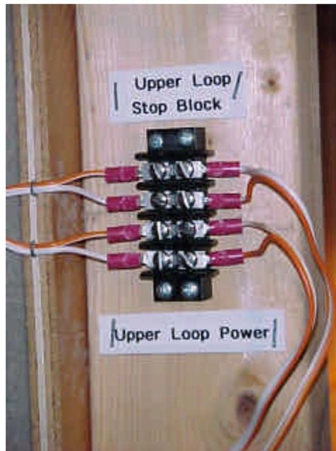
In this way, each node can handle up to 14 different connections to accessories. Eight accessories can be connected to the inside screw posts, and six more can be connected on top of the jumper strip to the outside screw posts.
