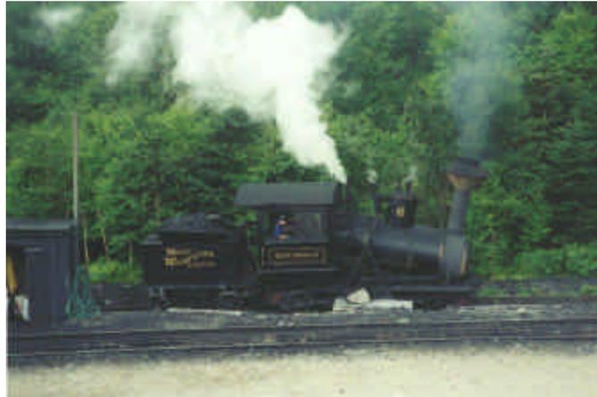
This railway has its own distinctively designed engines with tilted boilers and balloon smoke stacks. This is the world's first steam powered mountain cog train (1869) which travels up the world's second steepest railway track and includes grades up to 37%. This is the only railroad in the world built entirely on trestlework.
