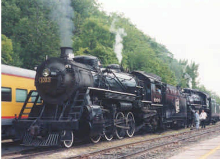
Northern Pacific #328 was built in 1905, by the Rogers Locomotive Works of Paterson, NJ, for the Northern Pacific Railroad. It is a 4-6-0 "Ten Wheeler" type and is hand-fired with coal. It was retired from service in 1955 and donated to the city of Stillwater, Minnesota where it sat in a park for many years. In the seventies it was restored to operating condition and subsequently leased to the Minnesota Transportation Museum.
